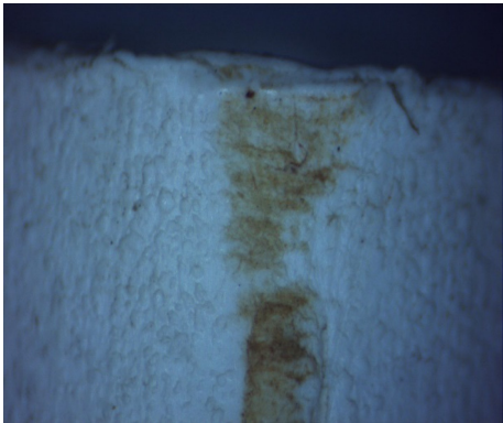
图 5 失效卡丁车座椅螺丝柱断裂起始区体视显微镜微观形貌照片 Figure 5 Stereomicroscope micrograph of failure karting car seat screw column's fracture initiation zone
